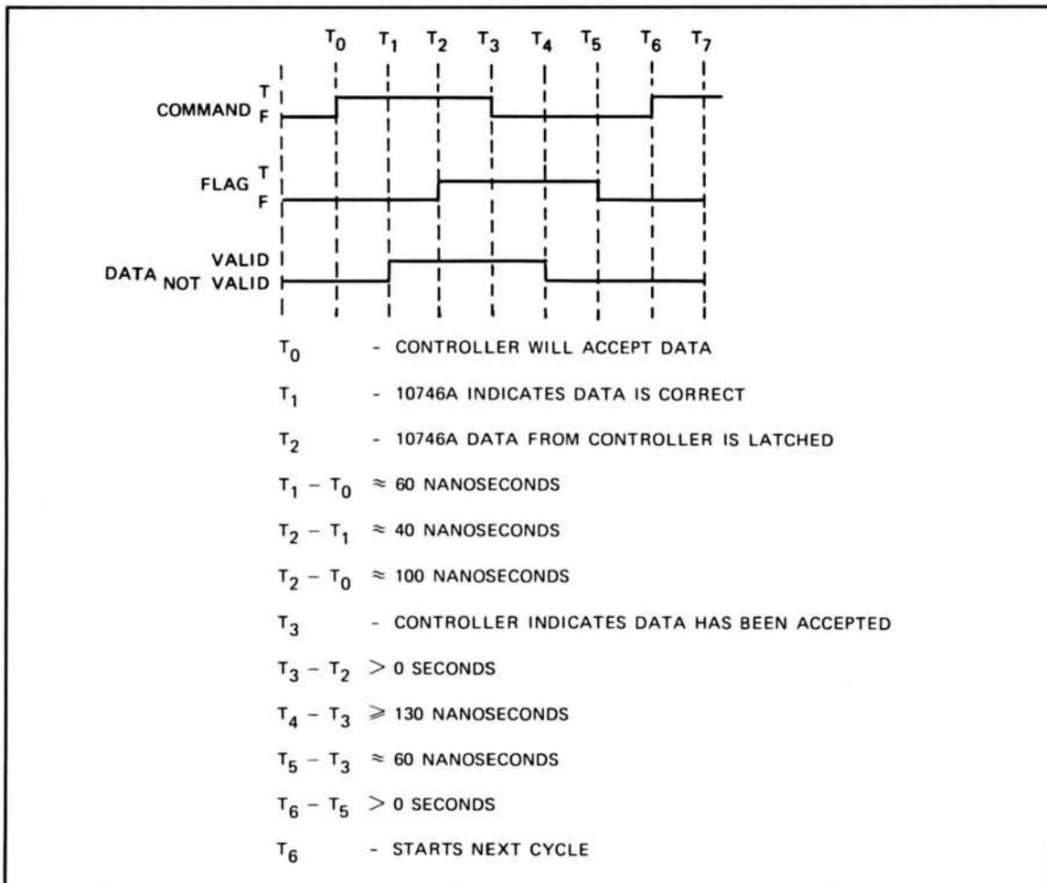
Figure 4-6. Instruction Sequence — Data to Controller from 10746A
