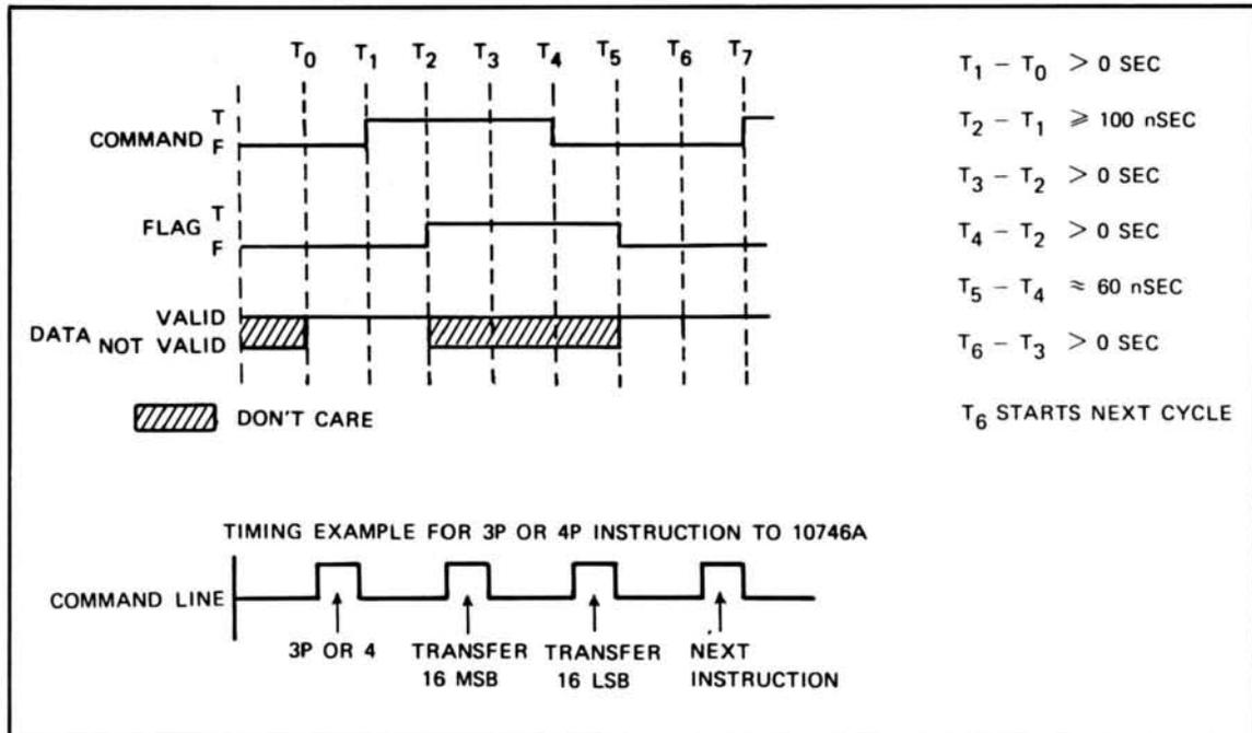
Figure 4-5. Instruction Sequence — Data to 10746A from Controller
