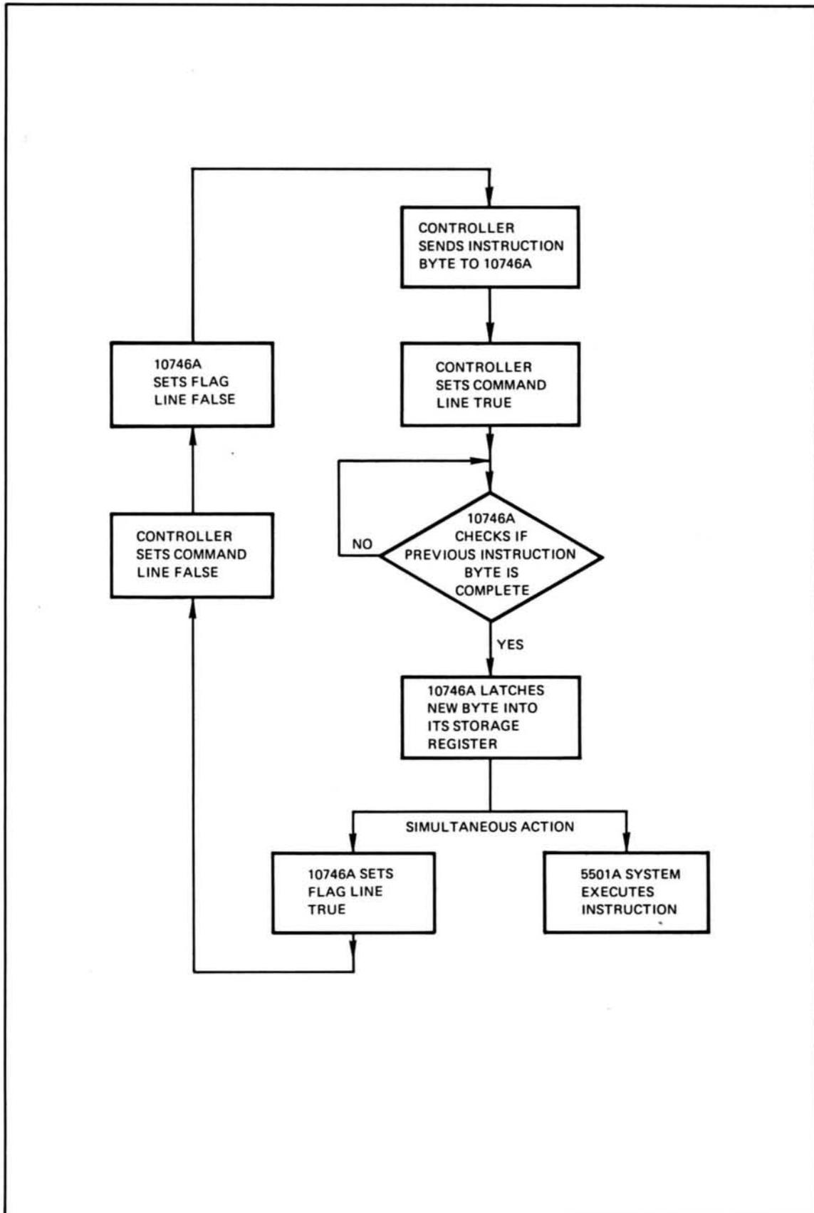
Figure 4-4. 10746A Controller Operation Flow Chart
